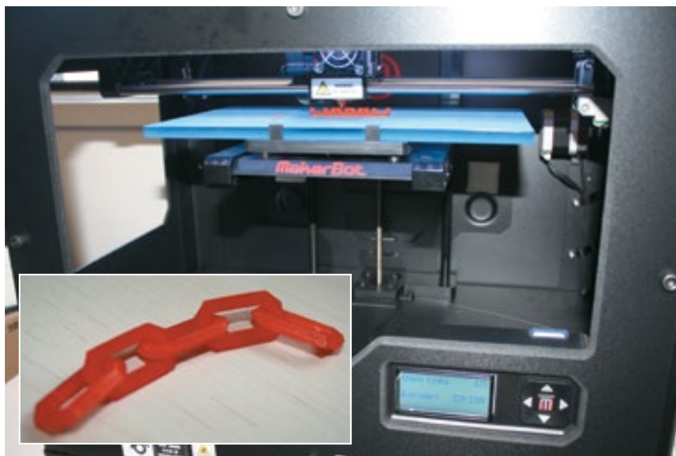
Chain link demo in mid-print, and the finished product (inset)
